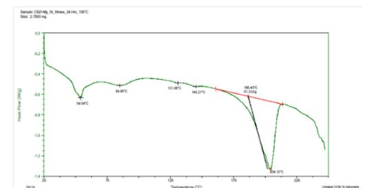
Figure 6. DSC thermogram of CBZ-MgStearate stressed sample.
