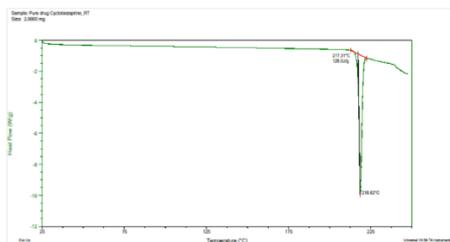
Figure 3. DSC thermogram of CBZ control sample.
