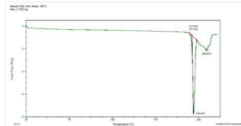
Figure 4. DSC thermogram of CBZ stressed sample.
